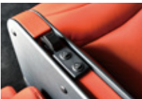
Controller for partition Controller for indirect lights (located on the floor and ceiling)
